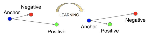
Fig. 1: Triplet loss visualisation [39]
